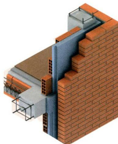
MUR I THJESHTË DHE MUR DOPIO ME PARET TERMIK AJRI / SINGLE WALL DOUBLE WALL DOUBLE WALL WITH AIR GAP
